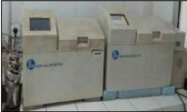
Gambar 3 : Bom Kalorimeter Parr 6200
